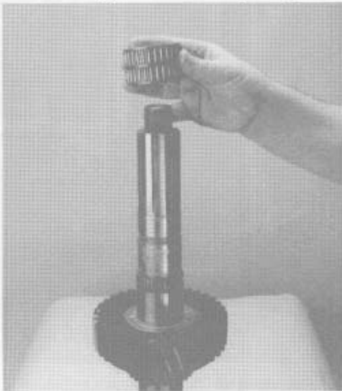
5. Install mainshaft reverse gear bearing.
