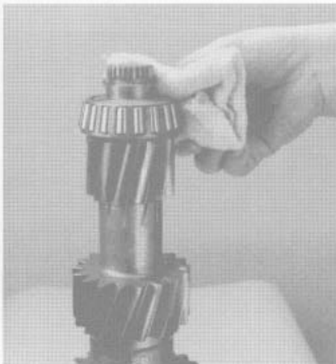
5. Heat and install the rear countershaft bearing. CAUTION: Do not heat the bearing above 275°F (136°C). If possible, use a heat lamp as the source.
