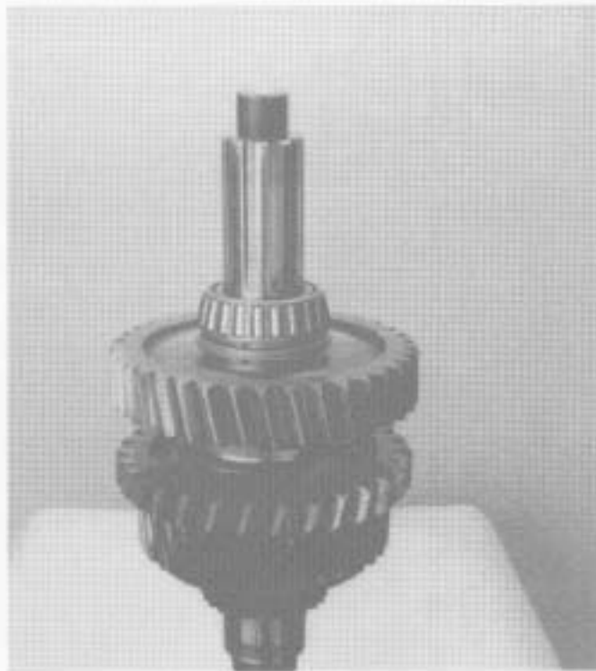
14. Reposition mainshaft in the vise so rear bearing is up.
