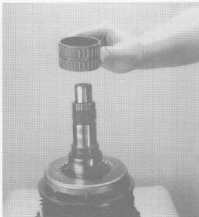
12. Remove the 3rd gear bearing.
