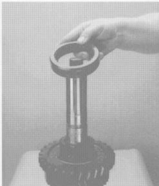
21. Remove the 1st-reverse sliding clutch.
