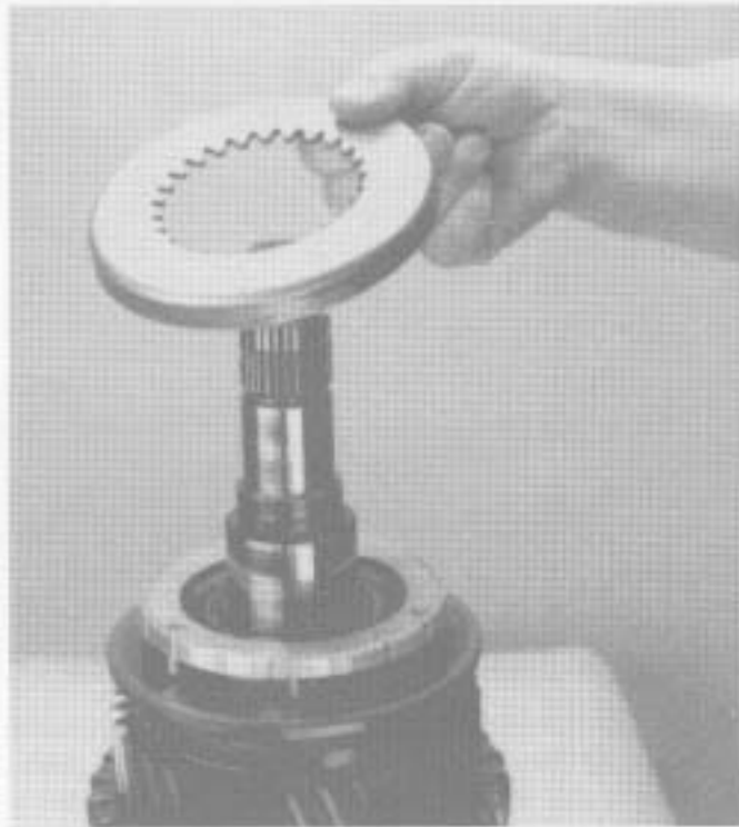
16. Install the mainshaft 3rd speed gear synchronizer cup as shown.
