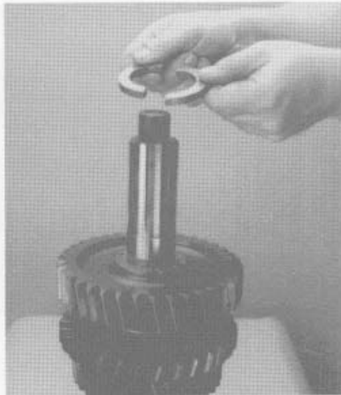
17. Remove the 1st gear split washer.
