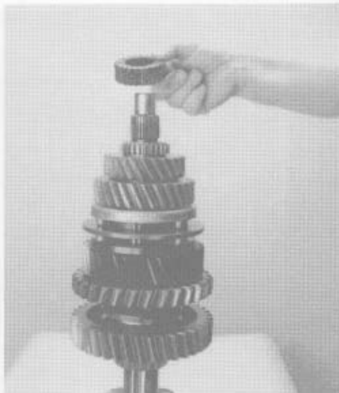
23. Install mainshaft 4th-5th speed clutch hub, machined surface facing up.
