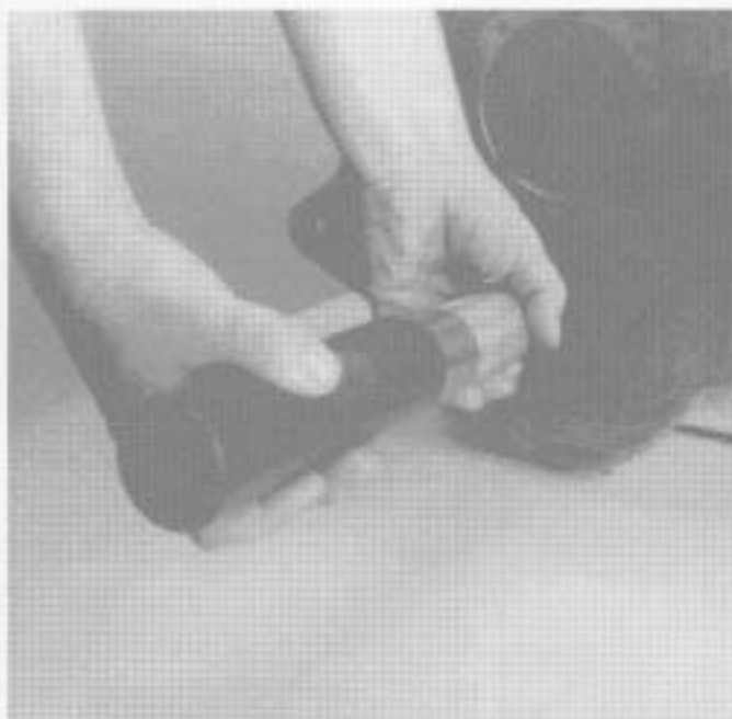
6. If previously removed, install the snap ring, countershaft front bearing race (from inside of case) and front case bore plug. Coat the outer diameter of bore plug with Loctite #510 before installing.
