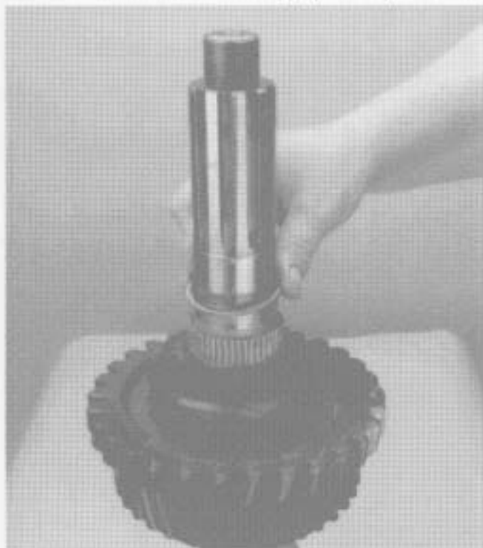
19. Remove the bearing rollers and spacers.
