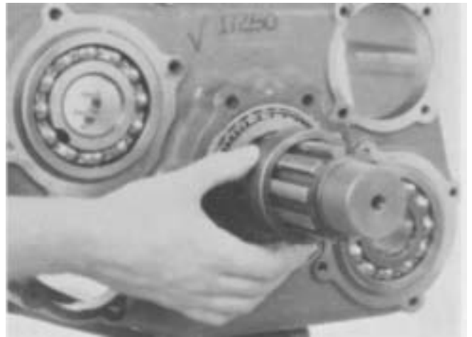
5. Slide speedosponder (or gear, depending on model) off output shaft.
