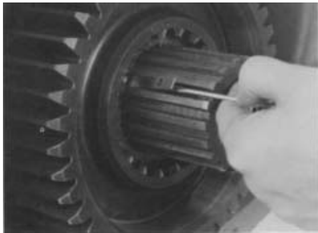
2. Remove the square key from the range mainshaft.
