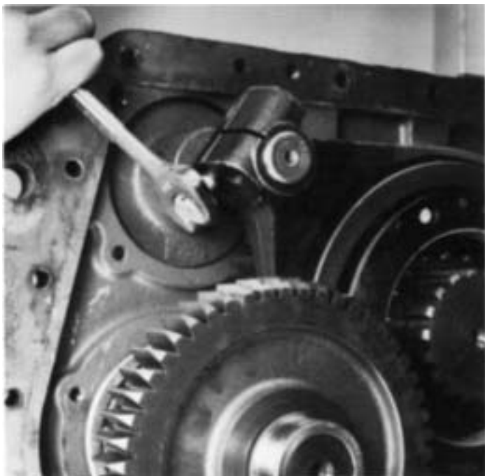
3. Cut lockwire and remove two yoke lockscrews.
