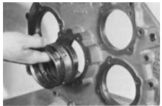
9. Remove the two bearing cups and outer spacer from the housing bore.
