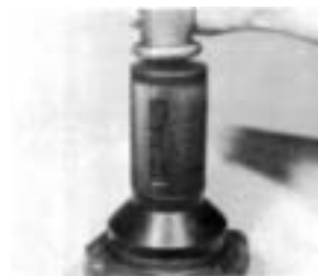
OIL SEAL DRIVER Print Number T-18088-37 Print Number T-18088-36 (RT-1110) Used to install the oil seal in the rear bearing housing.
