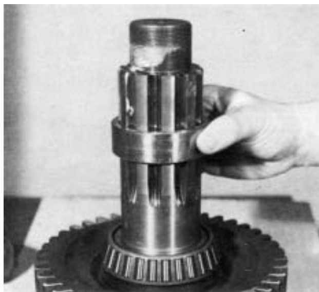
6. Install the bearing inner spacer on the shaft.
