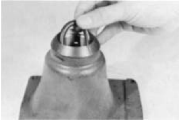
1. Install the O-ring in the top of the housing.
