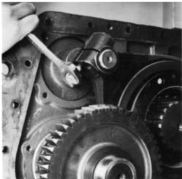
3. Cut lockwire and remove two yoke lockscrews.
