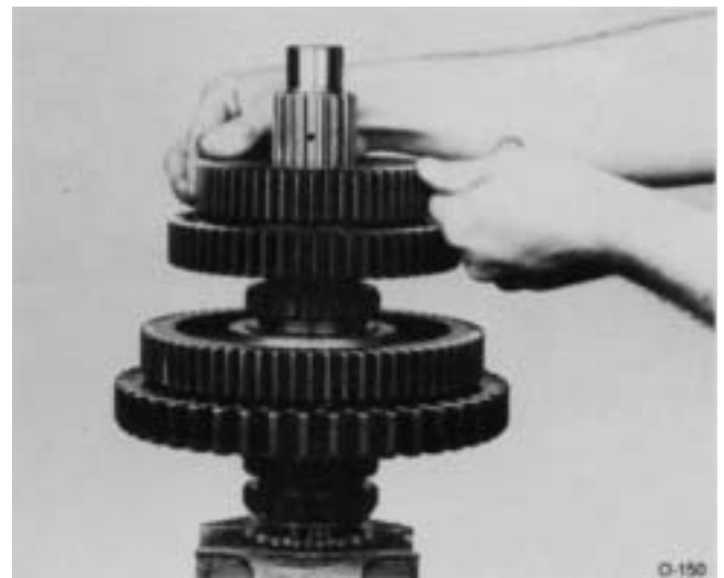
19. Install 4th speed gear, clutching teeth up, against 3rd speed gear.
