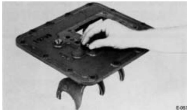
10. Remove housing from vise and install the three shift bar tension balls in bores in top of housing.
