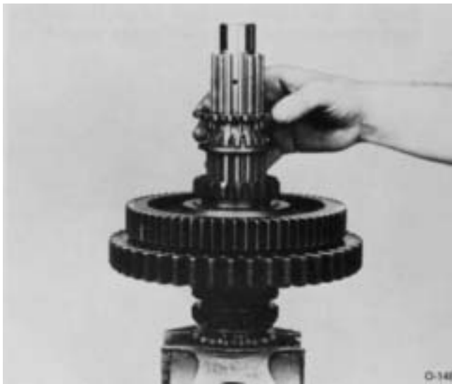
17. Install spacer against flat side of 3rd speed gear limit washer.
