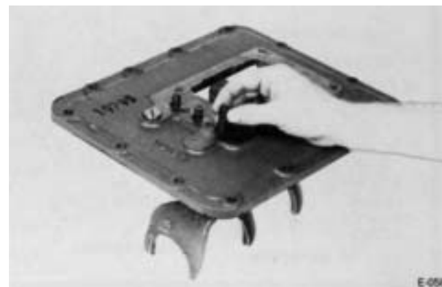
11. Install three tension springs in bores.
