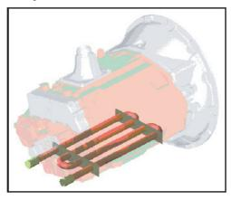
The engine coolant circuit will require 400 ml of coolant to fill the heat exchanger. Additional coolant volume is in the lines between the engine and transmission.
