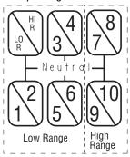
The shift pattern instruction label for this Lightning series transmission is available as Eaton Fuller part number 5586257.
