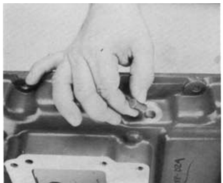
12. Install the reverse light switch pin in the shift bar housing.
