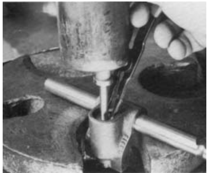
11. Place the shift yoke in a hand press. Depress retaining washer and spring and install the snap ring.
